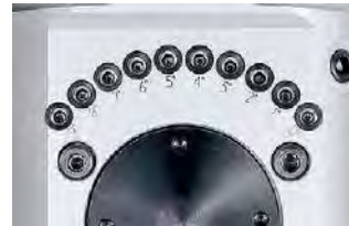
Indexing mechanism in 1° increments
