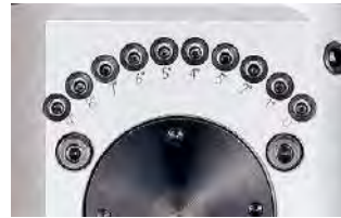
Indexing mechanism in 1° increments
