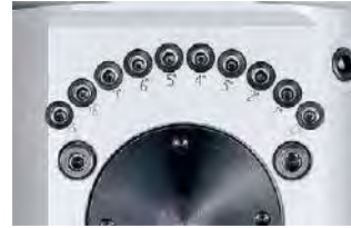
Indexing mechanism in 1° increments
