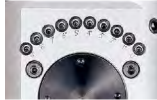
Indexing mechanism in 1° increments
