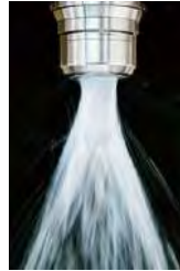
Flood Jet-Through Coolant
