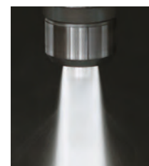
Peripheral coolant supply to cutting edge
