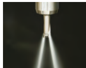
Rough Boring Through holes
