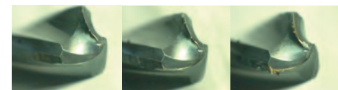
200穴 1000穴 2000穴 200 holes processing 1000 holes processing 2000 holes processing
