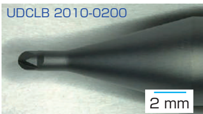
Tool #1 milled depth 3.5 mm.
