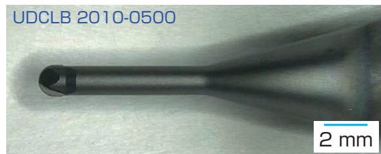
Tool #2 milled 131.9 \text{ mm}^3 in 76.5 minutes.
