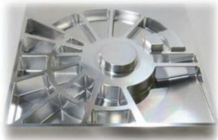
Work Size : 50 x 50 x 50 mm Coolant : Water Soluble
