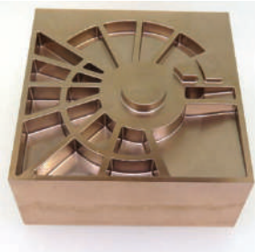
Work Size : 50 x 50 x 50 mm Coolant : Oil Mist
