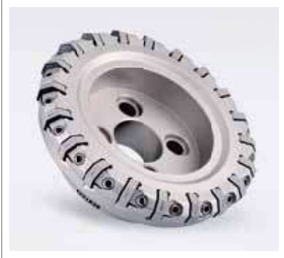
AFM45-XN09-W milling cutter with heptagon inserts, extra close pitch with wedge clamping, combined with heat resistant CVD coated inserts. The ideal choice for cast iron rough milling.
