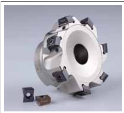
ASM90-LN09/LN13 square shoulder milling cutter with 4 cutting edge tangential inserts with helical edge profile. The reliable cutting edge can adopt 30% higher f_z , higher metal removal rate and productivity.
